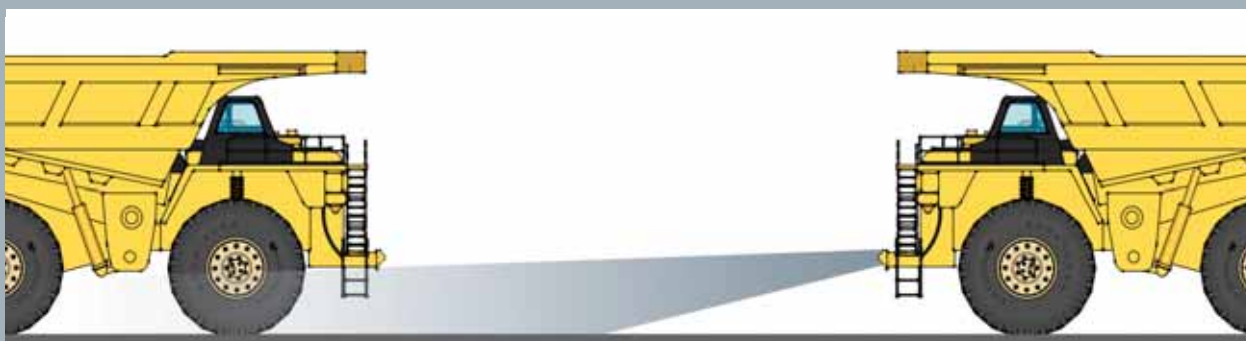
The ZEROGLARE optics ensure light vehicle operators are not blinded by oncoming Haul Trucks lighting systems
