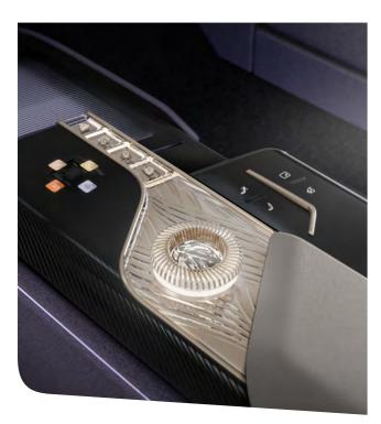
**Thermal comfort** featuring large surface lighting and injected radiant panel heating that creates an efficient comfort solution that utilizes 30% less kWh, to improve EV range.
